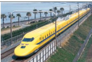
"Dr. Yellow" checks the condition of the track and overhead power supply wires.
